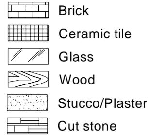
Figure 6. Examples of material symbols in elevation
