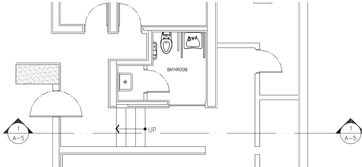
Figure 13. Section symbols used on the plan view
