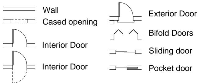
Figure 7, Walls & doors symbols in plan view
