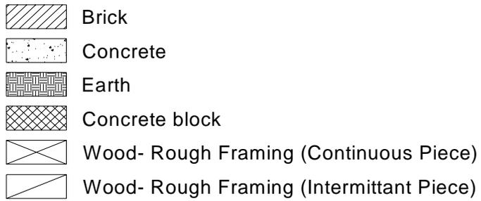
Figure 5. Examples of material symbols in section
