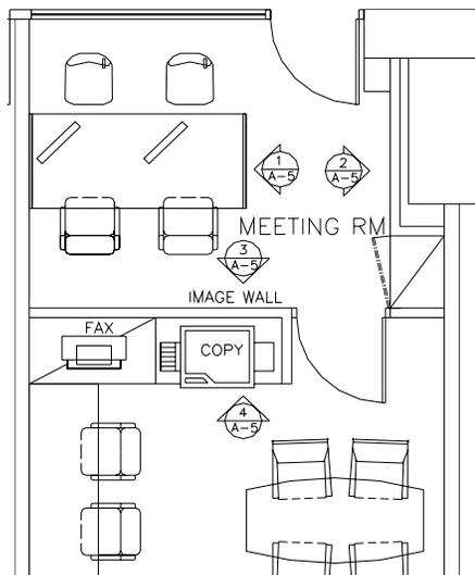
Figure 16. Elevation symbol used on the plan view
