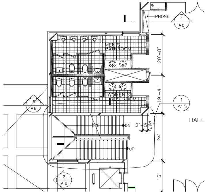
Figure 19. Detail symbol used on the plan view
