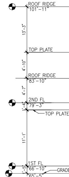
Figure 42. Dimensioning exterior elevations 2
