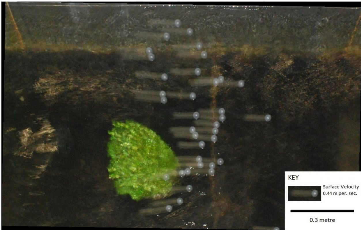
Figure 7 Scaled orthophoto showing velocity vectors in the XY plane, flume application
