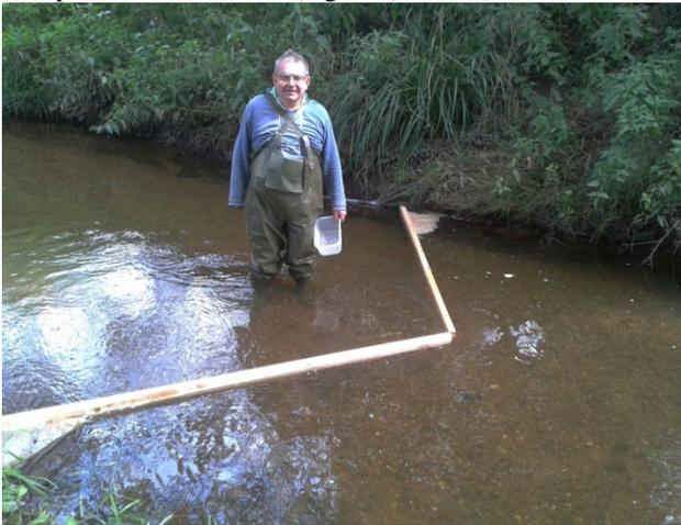
Figure 5 Two hinged wooden spars used for collecting spheres
