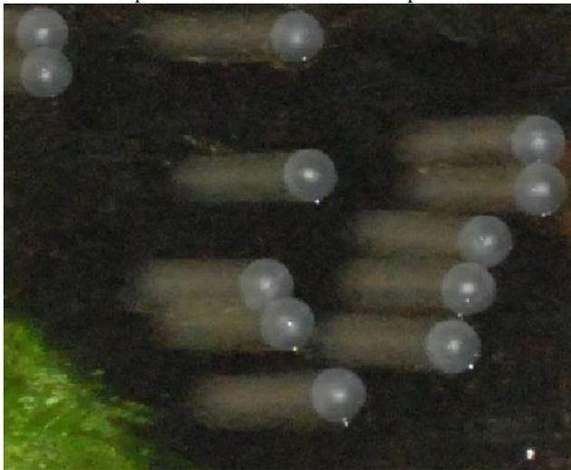
Figure 2 Deliberately blurred targets for velocity determination
