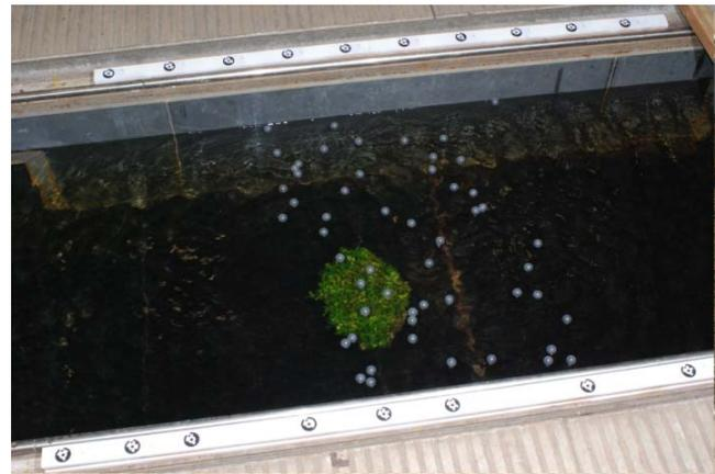
Figure 4 Control layout for laboratory application with evenly distributed “sharp” targets
