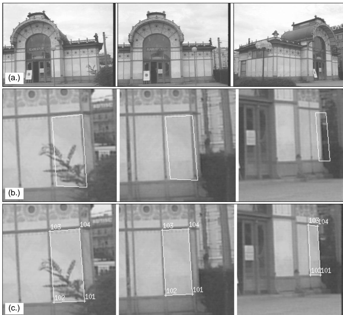
Figure 4: Performance of 3D-FEX routine of a single feature in three images simultaneously. (a.) images from a sequence (b.) initial 3D position of feature from approximate model, projected into image planes (c.) final 3D position of feature after 5 iterations, projected into image planes
