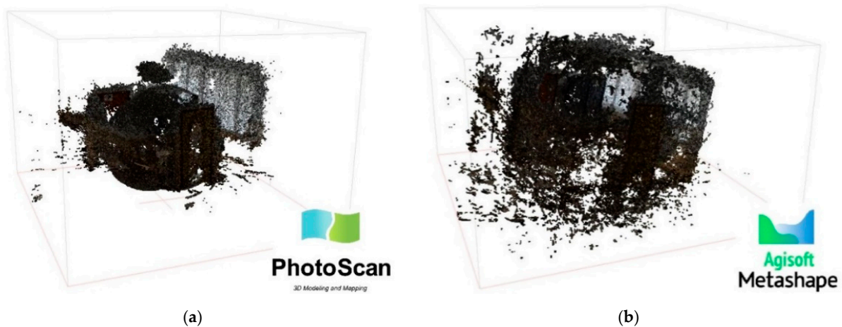
Figure 3. Results of point cloud (room of the laboratory) processing in Agisoft Photoscan (a) and Agisoft Metashape (b).
