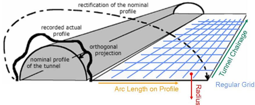
**Figure 2: Surface unwrapping for image-based tunnel surface representation**
