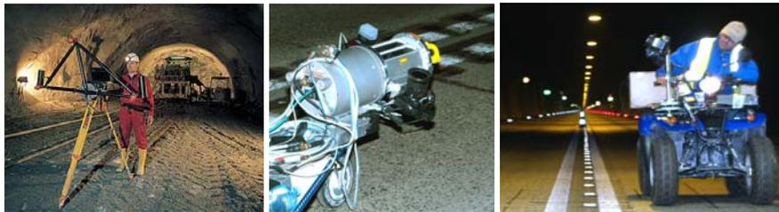
**Figure 3: Left: Photogrammetric data acquisition. Middle: Simultaneous Laser-Scanner and image data acquisition. Right: Image acquisition to update texture information of existing tunnel surface reconstructions**
