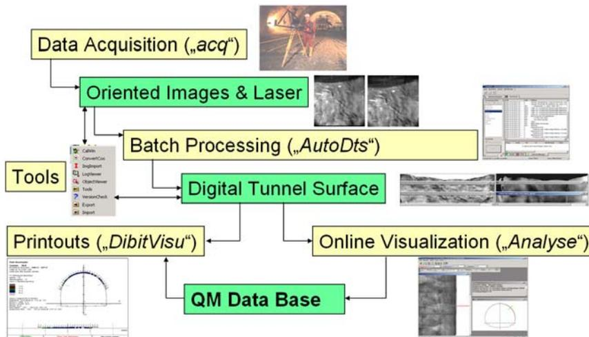
**Figure 1: Major components of tunnel reconstruction system Dibit**
