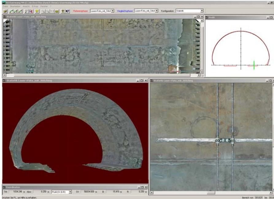
**Figure 4: Analyse Module, used for interactive tunnel surface visualization. Clockwise from top left: Overview (RGB ortho overlay) of 10 m chainage, profile display, enlarged texture part with 4mm resolution, rendered 3d plot**
