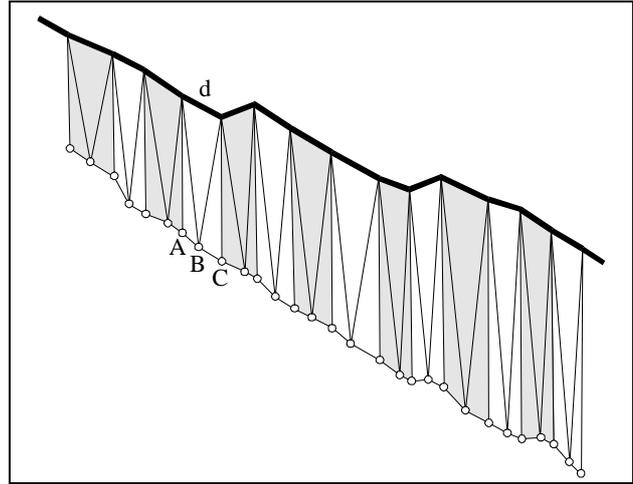
Figure 1. Breakline and points forming 'vertical' triangles.
