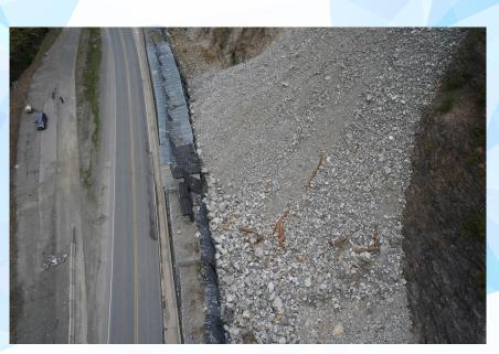
Aerial view of a debris slide catchment area. This photo shows the catchment area before the contractor has removed the debris and is one of many that will be imported into PhotoModeler to calculate the total debris volume of the slide.
