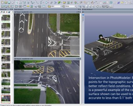
Intersection in PhotoModeler. Blackburn said, "In creating the line work and points for the topographic survey, I experimented with creating surfaces to better reflect field conditions. While this graphic is not used for the design, it is a powerful example of the capabilities of this software. Any portion of the surface shown can be used to create three dimensional points and linework accurate to less than 0.1' both vertically and horizontally.
