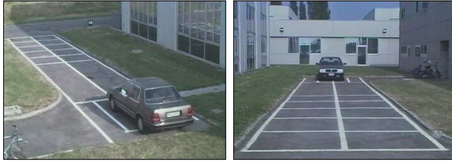
Figure 6: The grid used for the vision system calibration and the ARGO vehicle
