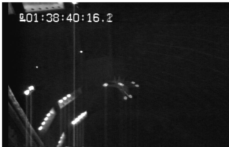
Figure 5.10 Image trails of intense light sources caused by smearing in a frame transfer CCD sensor (from Shortis and Snow, 1995).
