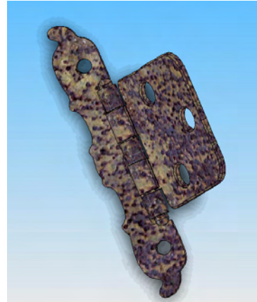
Figure 20. Applying a Rust Finish to the Reverse Engineered Bracket
