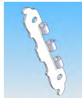
Figure 8. A Linear Pattern Was Used to Duplicated the Center Part of the Hinge
