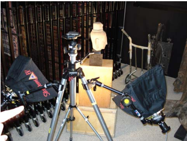
Fig.7. Illumination system used for the texture mapping.
