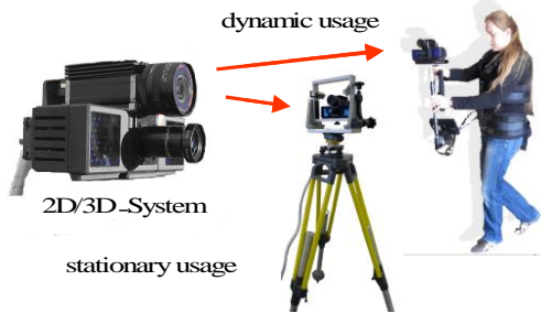
Figure 1 Dynamic usage of the 2/3D camera system (for recording) and stationary usage (for surveying and recording)
