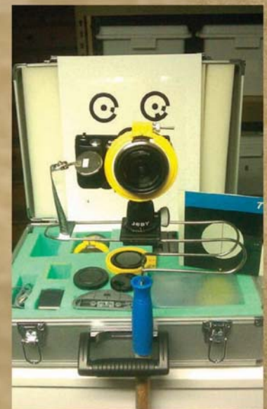
Figure 2. The camera in front of its case. Note the yellow lens clamp. Also note the small mirror that allows shutter actuation from below via infrared remote. Behind the camera is one of the 16 white calibration panels.
