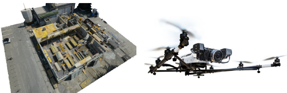
FIG. 2. UAV and structure from motion. In project Construct from Graz University of Technology, an AscTec Falcon 8 UAV (right) was used to obtain 242 images. The resulting 3D model used structure-from-motion software where each object point was shown on an average of 19 images. © Christian Mostegel – ICG Graz University of Technology.
