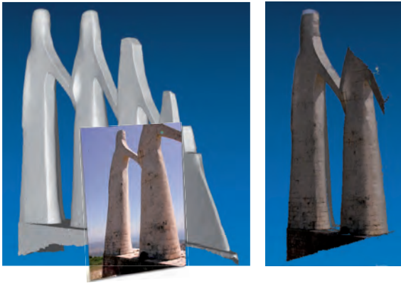
Figure 5: Example of the input and output of the photogrammetric texture mapping module created in Matlab
