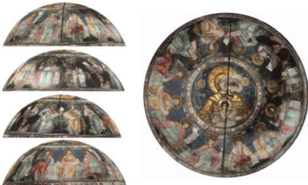
Figure 9. Orthophotos of the circular dome T5L2, left the lateral projections and right the ground projection. ( R= 1.94m , \sigma_R=2.3cm )
