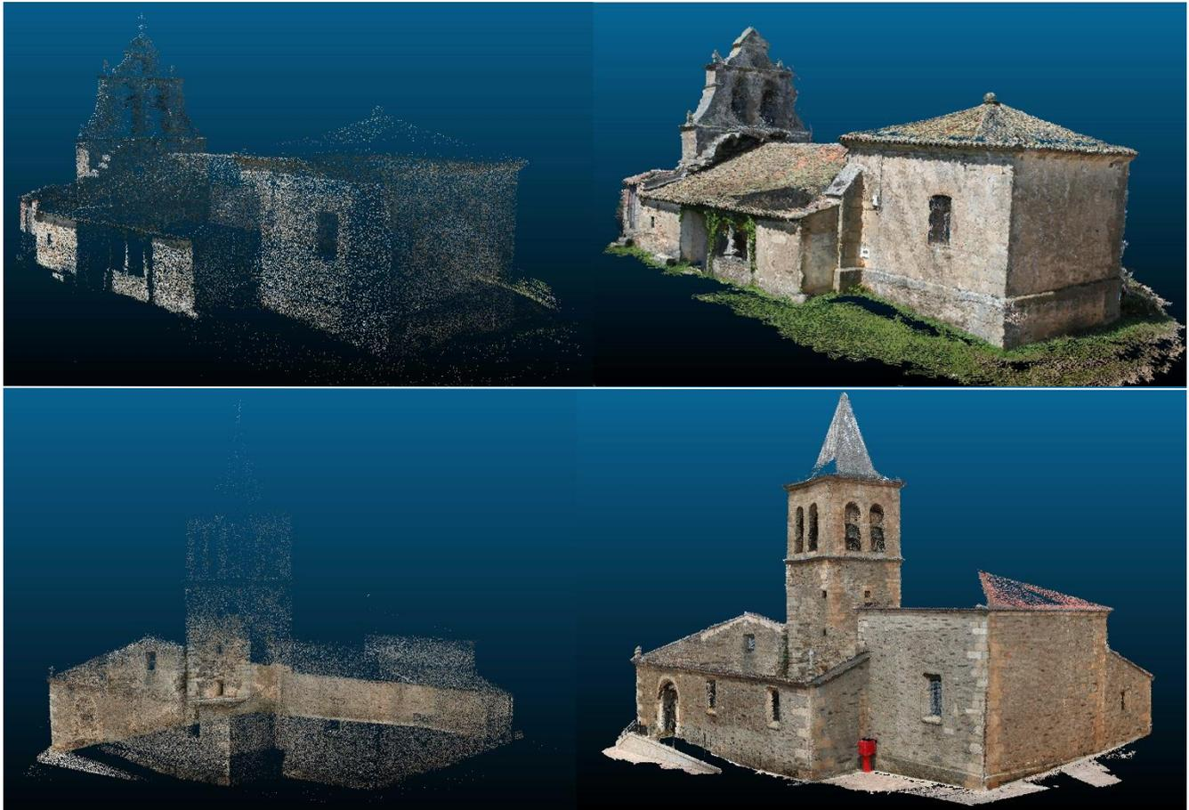
After removing noise from the images, the point cloud was divided into sections in order to outline the ground plan and export it to a CAD program, so as to draw the geometry. Moreover, we obtained the orthogonal profiles of the façades and then processed them with a CAD program to get the final product (Figure 6).
