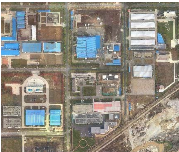
Figure 9. DOM of the test area generated by image sequences
