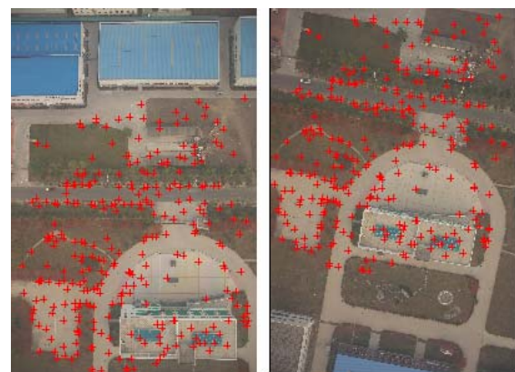
Figure 8. Matched conjugate points of images of adjacent strips
