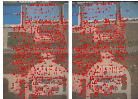
Figure 7. Matched conjugate points of a stereo pair
