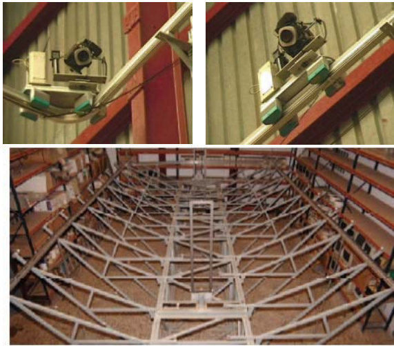
Figure 18: Camera shuttle in different measuring positions (top), and space frame with targets on cantilever arms and receiver supports (bottom).
