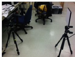
Figure 1: Data capture of a white planar Spectralon target using the Microsoft Kinect.
