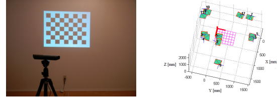
Figure 8: (a) Experimental design for calibrating the Kinect. (b) Network configuration of the calibration.
