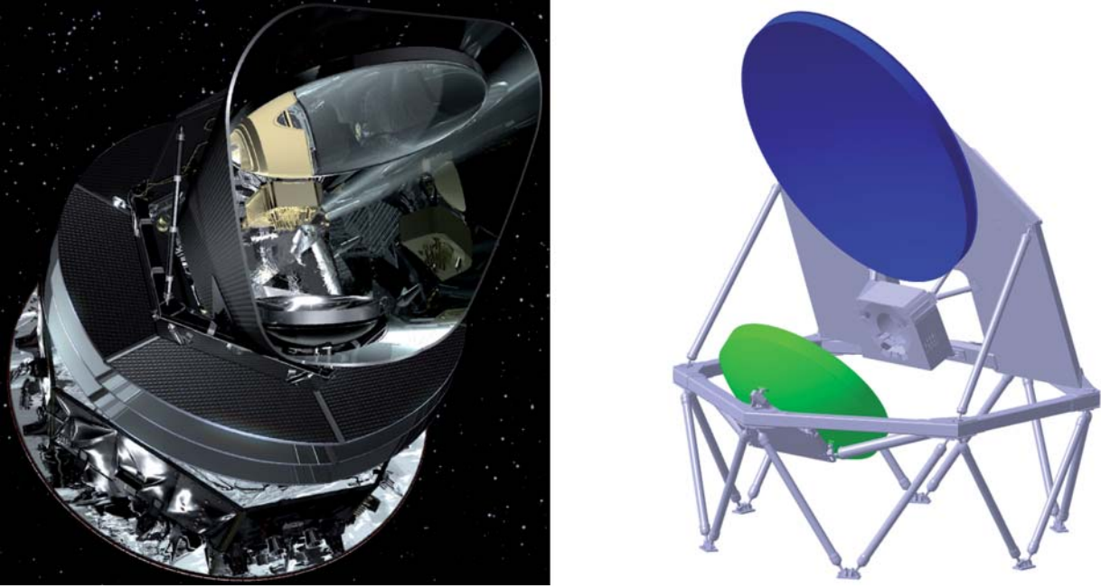
Figure 1: Planck Telescope (left). The telescope structure (right) with primary reflector (top) and secondary reflector (bottom). Copyright ESA, right view courtesy Thales Alenia Space France.
