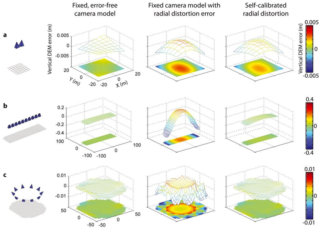
**Figure 4.** Convergent imaging geometries strongly reduce systematic vertical DEM error in simulations of (a) a single image pair (b) an image strip and (c) an orbiting camera scenario. See text and Figure 2 caption for more details. This figure is available in colour online at [wileyonlinelibrary.com/journal/espl](http://wileyonlinelibrary.com/journal/espl)
