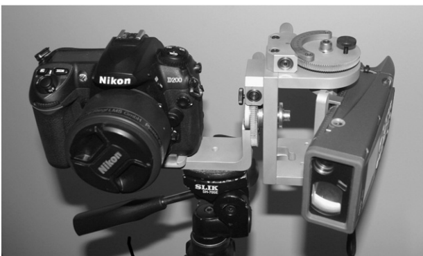
Fig. 1. View of the measuring system with their different elements: laser distancemeter, digital camera and aluminium support.
