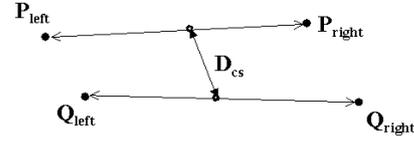
Figure 2: The disparity gradient between two correspondences ( $\mathbf{P}$  and  $\mathbf{Q}$ ) in image left and right.
