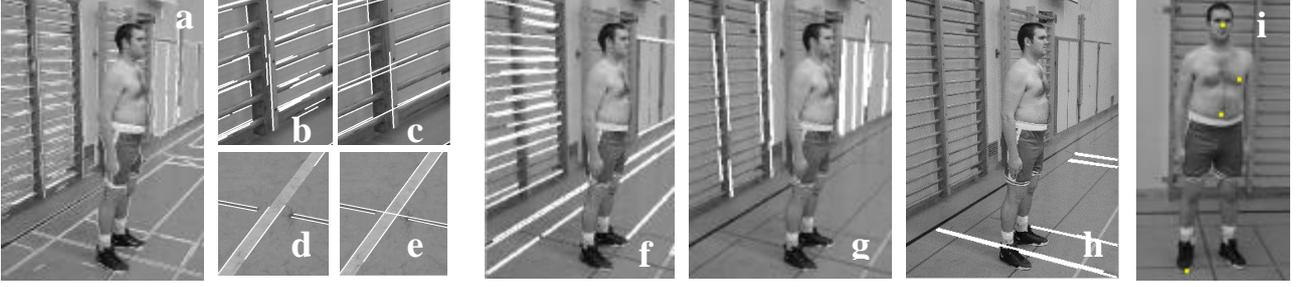
Figure.5: Extracted lines with Canny operator (a) and merged segment (b-c, d-e). Aggregated lines classified according to their direction (f,g,h). 4 control points measured manually on the body and used for the adjustment (i)
