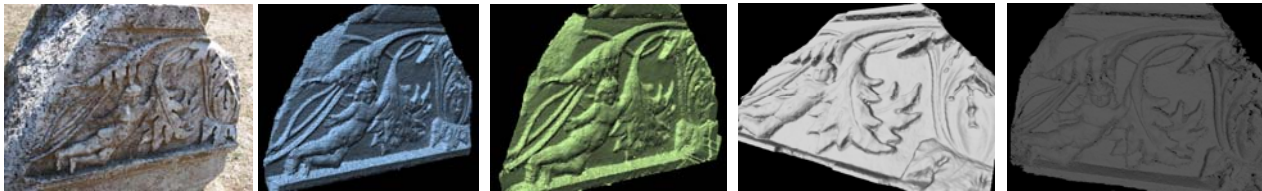
Figure 3: Stone example, modeled from 3 images: results respectively from NGATE, ATE, ARC 3D and SAT-PP.
