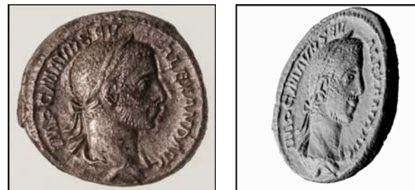
Figure 6: (a) 2D image of a Roman Denarius, (b) acquired 3D model of the same coin (visualized without texture).
