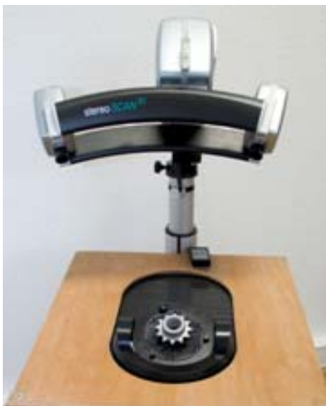
Figure 1: Setup with stereoSCAN-3D-HE system and rotation/tilt table
