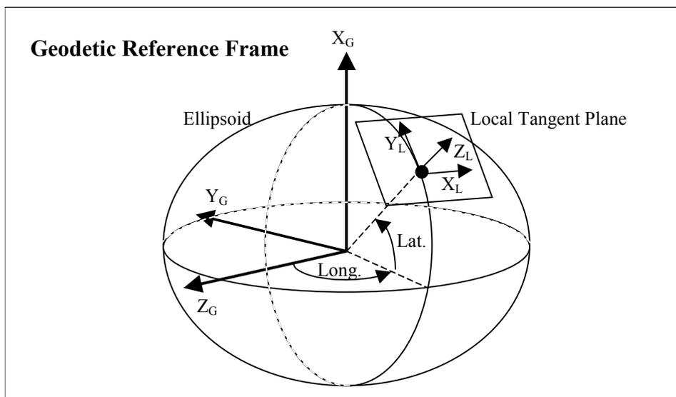
The Heading, Pitch, Roll rotations can be applied to transform the raw image to the correct location on the Local Tangent Plane. Aligning the image axes to the aircraft axes is usually quite trivial, and can involve swapping X and Y, changing the sign on one or more angles, and applying calibration offsets. After that, the Heading, Pitch, and Roll rotations are applied to map the raw image into the Local Tangent Plane.
