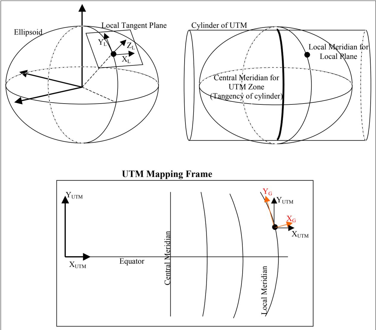
The reprojection between a Local Plane, referenced to ECEF locations, and a UTM projection, are complex geodetic calculations. At the moment, OrthoEngine and most other photogrammetric packages do not have this capability. The PCI OrthoEngine team is in the process of adding support for this transformation, so that Heading, Pitch, Roll data can be used directly.
