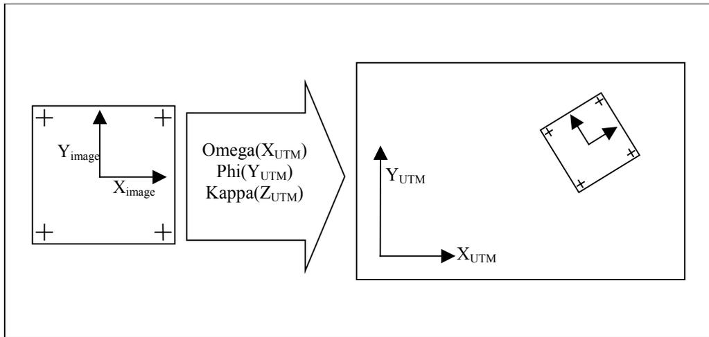
Most GPS/INS sensor providers have developed post-processing software to perform the complex geodetic transformation from Heading, Pitch, Roll to Omega, Phi, Kappa. Please refer to POS/EO from Applanix, or your own INS/IMU provider for additional information.
