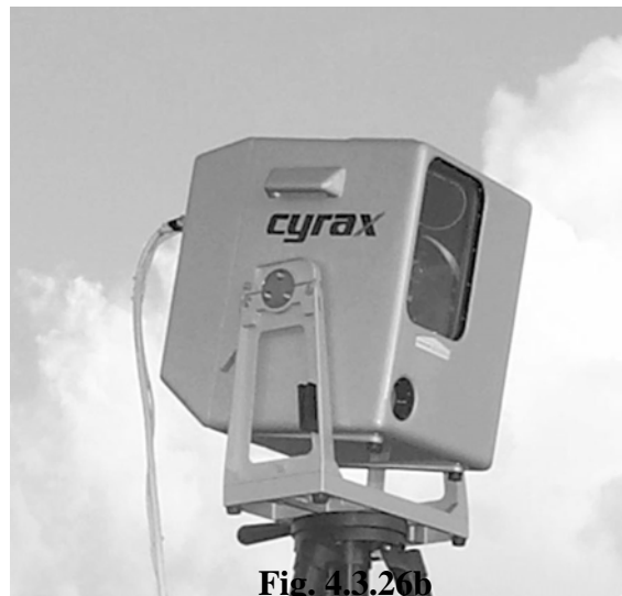
Fig. 4.3.26b A laser scanner using Lydar technology and the "point cloud" generated by it.
