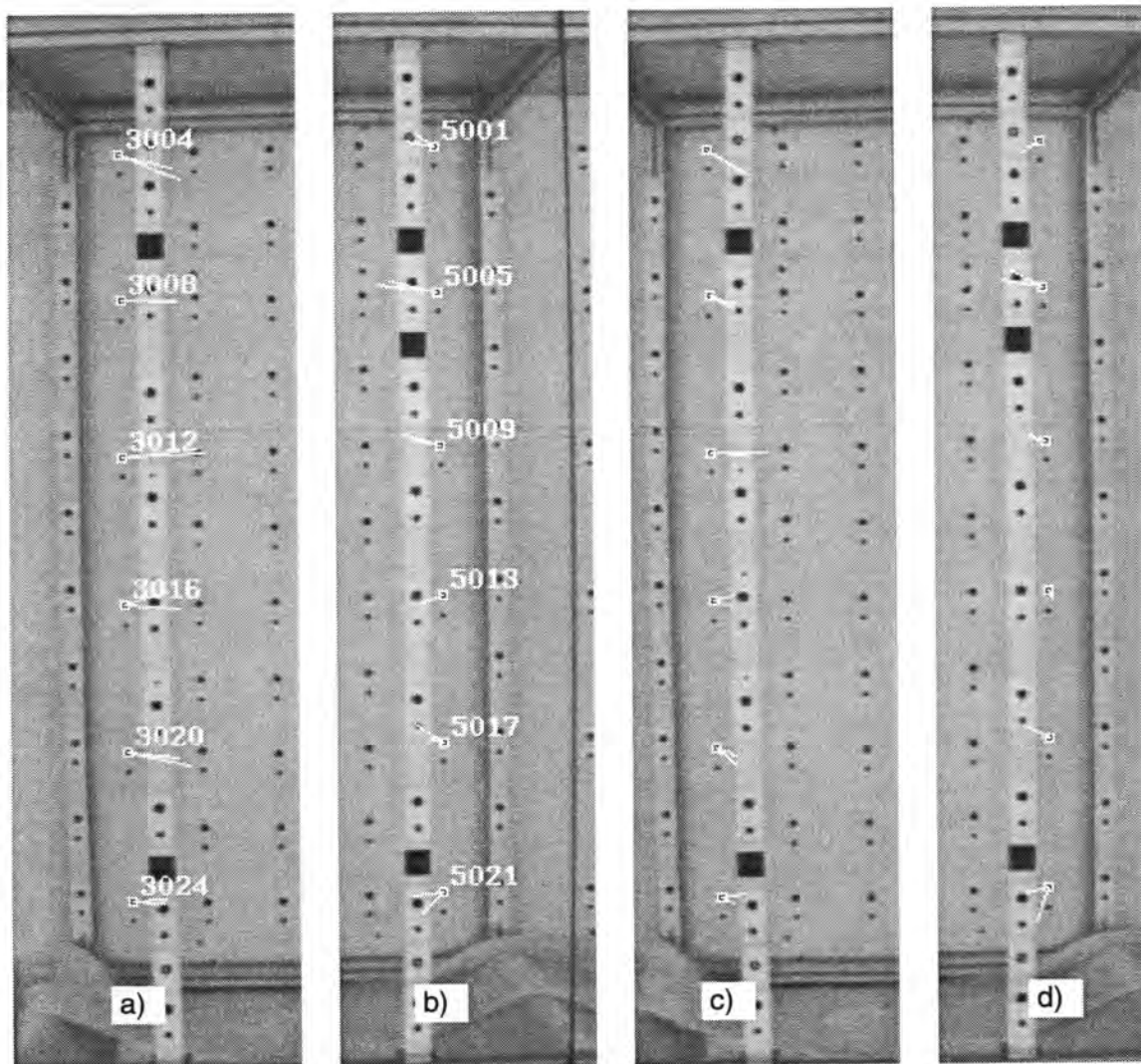
Figure 6.36 Displacements for 7 x 7 template (a and b) and 5 x 5 template (c and d) for left and right columns of targets.
