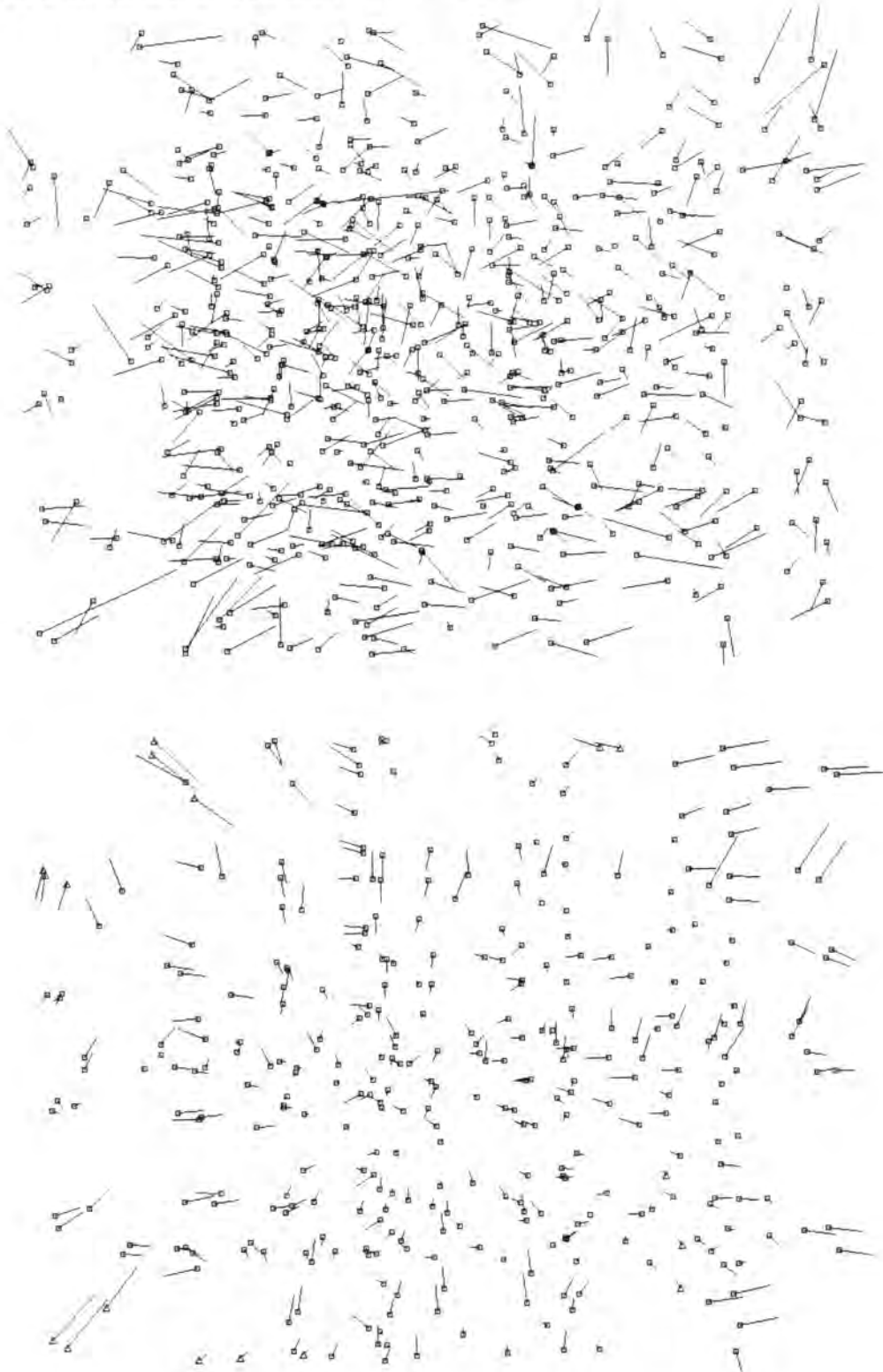
Figure 7.30 Residuals (top) and checkpoint differences for images taken at station 15xx of version cv611.
