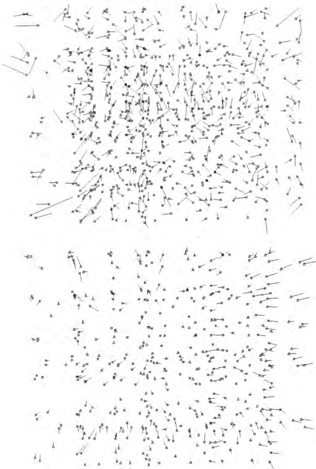
Figure 7.17 Residuals (top) and checkpoint differences (bottom) for images taken at station 15xx of version cvp243.
