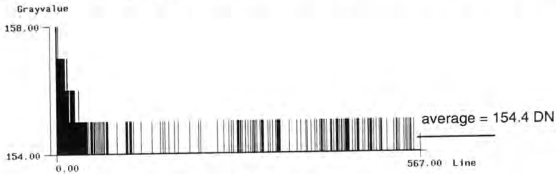
Figure 4.2 Cross-section through first 200 lines of an image showing typical errors with wrong DC-restoration.
