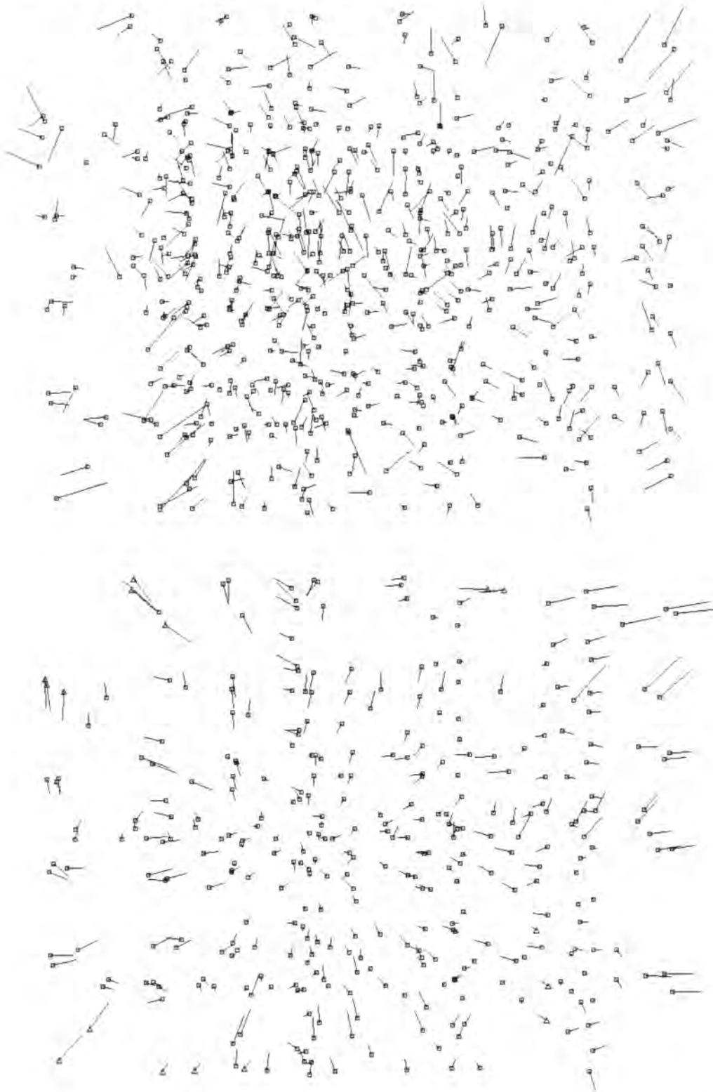
Figure 7.24 Residuals (top) and checkpoint differences (bottom) for images taken at station 15xx of version cvp611.
