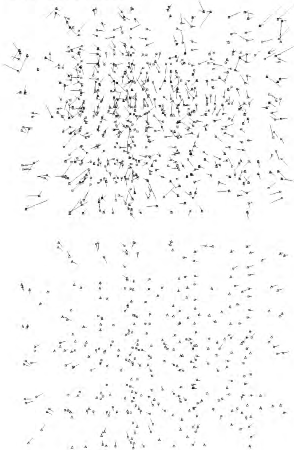
Figure 7.22 Residuals (top) and checkpoint differences (bottom) for images taken at station 15xx. of version cvp601.
