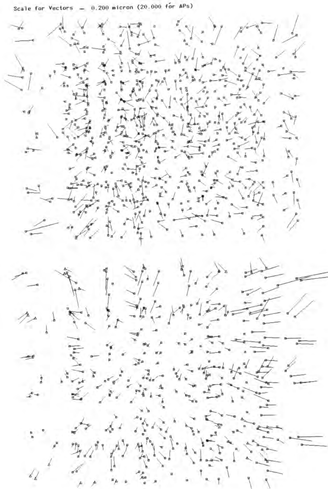
Figure 7.14 Residuals (top) and checkpoint differences (bottom) for images taken at stations 15xx of version cvp221.
