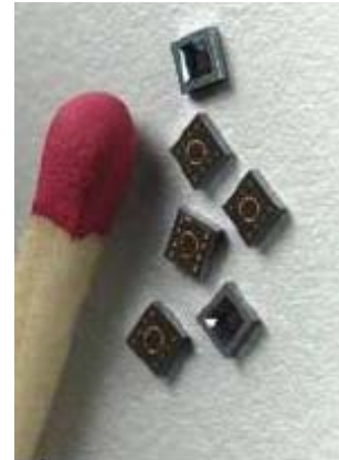
Figure 16. MEMS accelerometer sensors placed to monitor the dynamic of the structure
