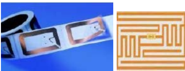
Figure 15. RFID sensors placed on basic elements for their automatic identification
