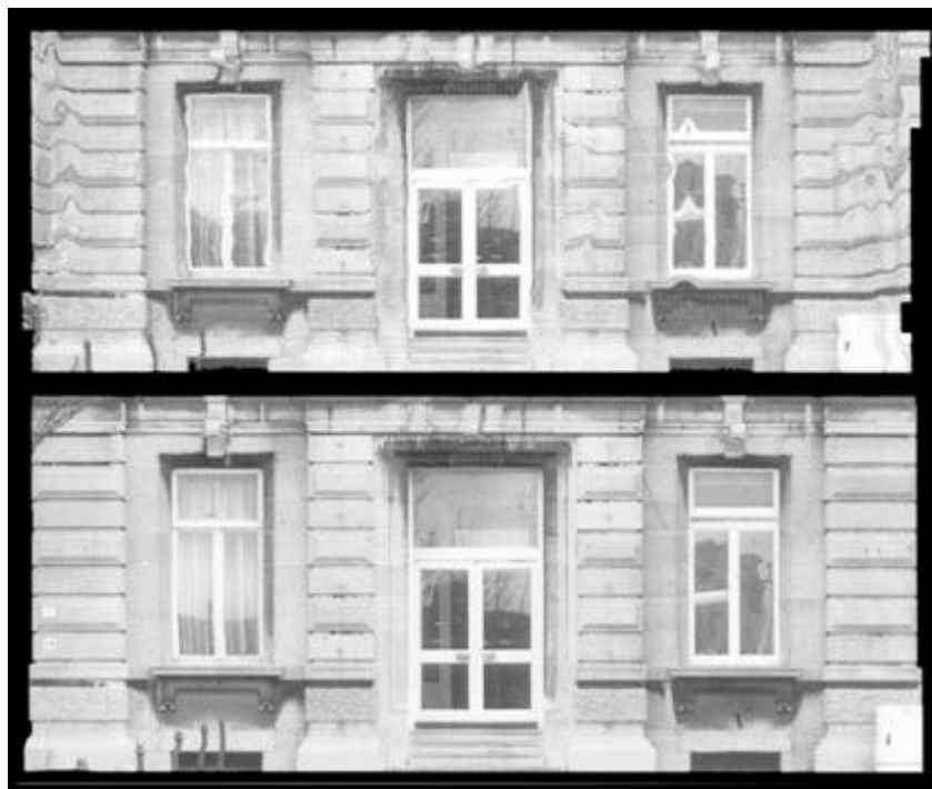
Figure 3 : Orthophoto from laser scanner before and after editing
