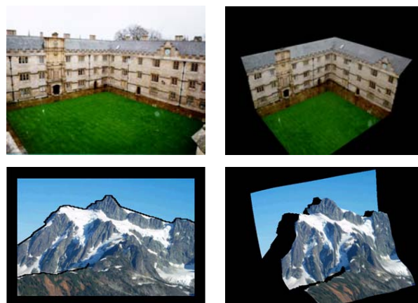
Figure 8: Two example of 3D reconstruction from a single image. Upper: 3D model of a building reconstructed using vanishing points and straight lines information [Criminisi et al., 1999]. Lower: Landscape 3D model reconstructed by [Zhang et al., 2001] using specific constraints on the shape of the scene.
