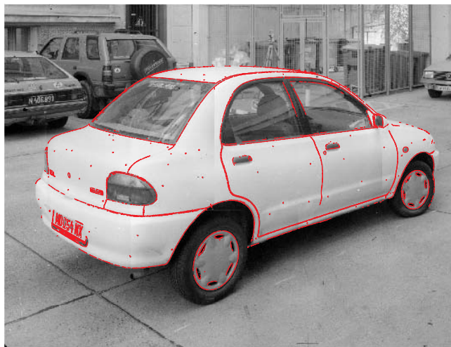
Figure 4: results of edge detection in one of the images. The regions outside the car body have been masked.
