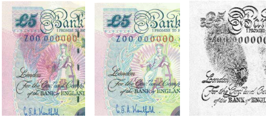
Figure 8: An example of removing the non-periodic background from an evidence mark. The evidence mark (a) is registered geometrically and photometrically to a sample image of the background (b) before being subtracted (c).
