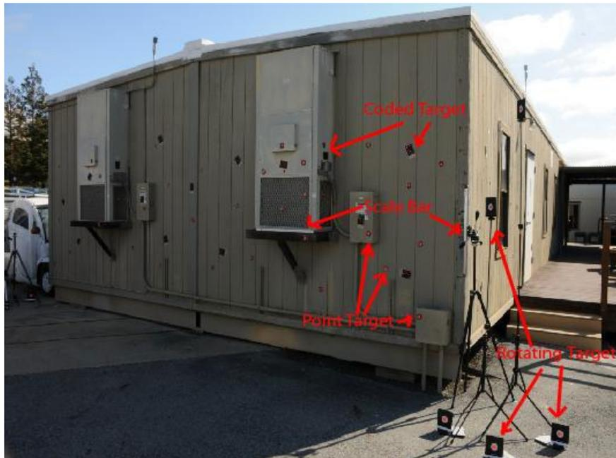
Figure 3 Complete target network on a façade.
