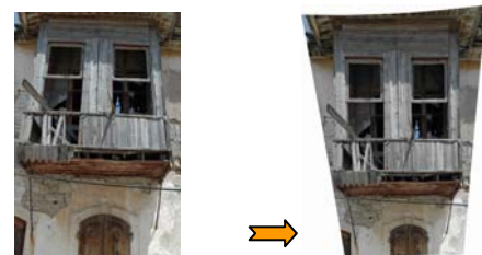
Figure 4. An original photograph and its orthoimage
