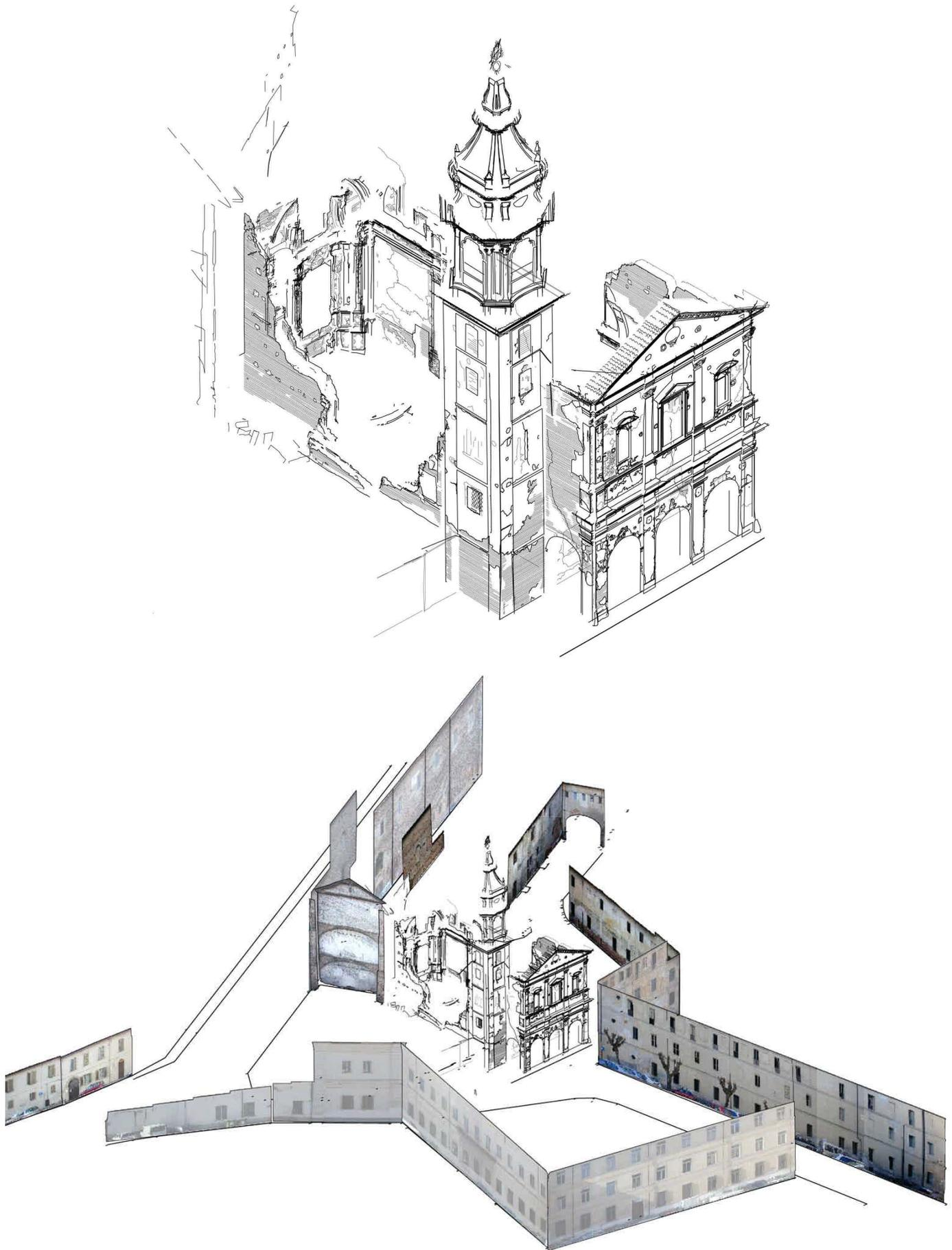
Figure 6. 3D models generated by the use of plotting and rectification results (drawing by Paolo Piumatti)
