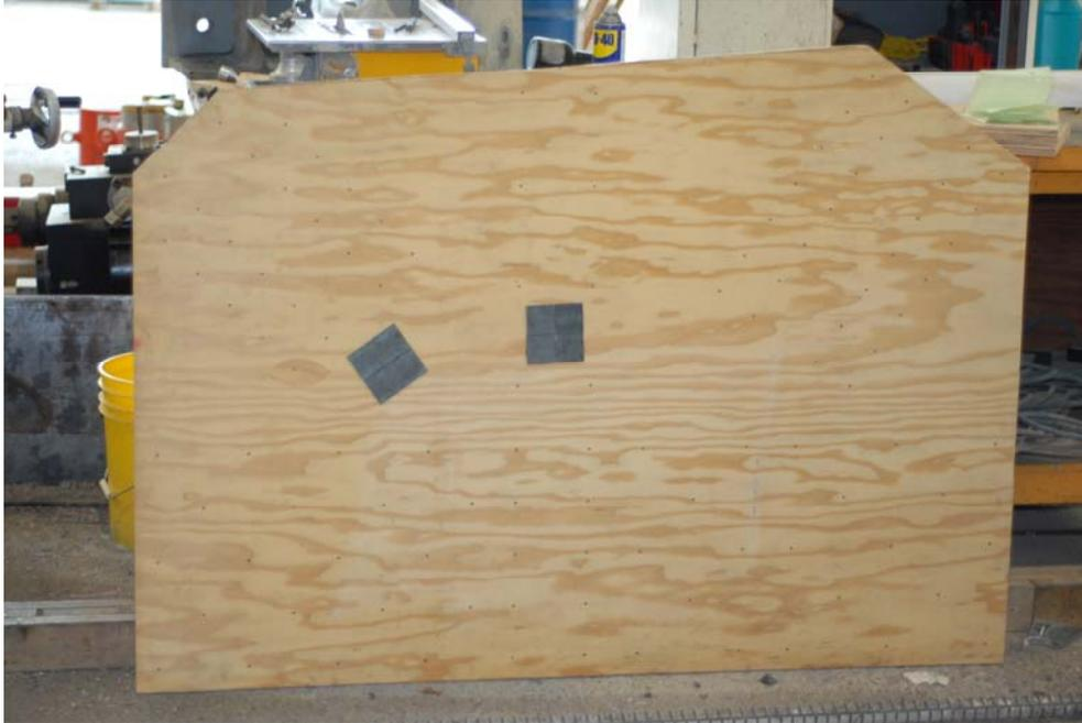
Figure 4.2: Mock gusset plate with steel plates to permit magnetic target attachment.
