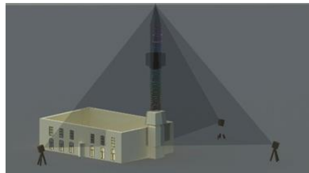
Figure 5. The scanning geometry from three points.
