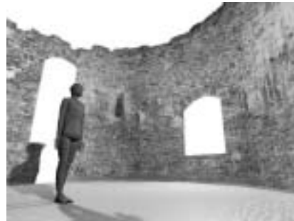
Fig. 6: a simple 3D model using a cylindrical orthophoto as texture.
