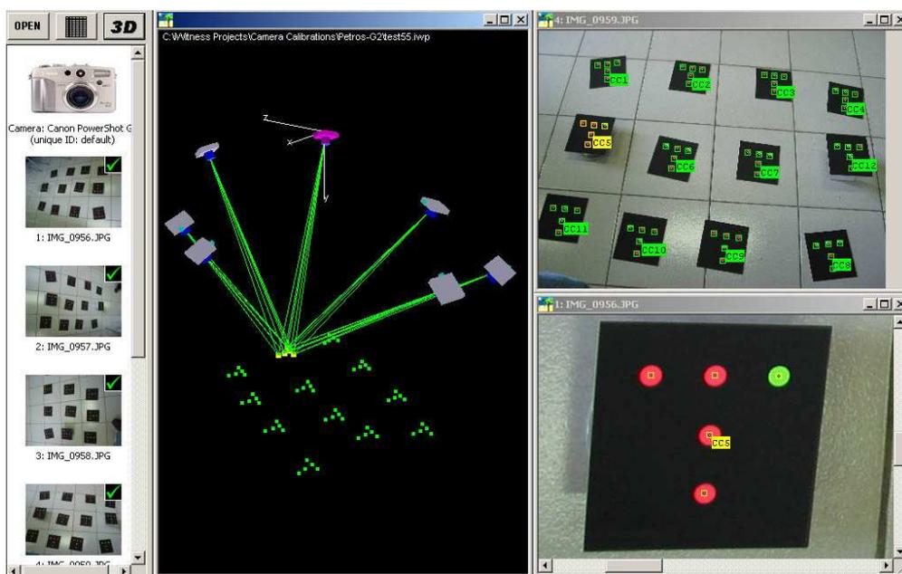
Figure 6. Automatic camera calibration in *iWitness*; note array of 12 colour coded targets.
