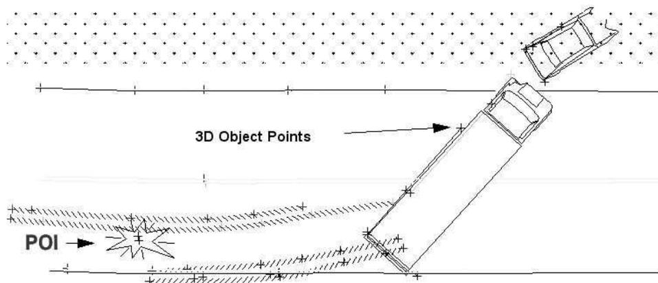
Figure 1: Example CAD drawing for AR illustrating object features of interest (courtesy of DeChant Consulting Services – DCS [2]).
