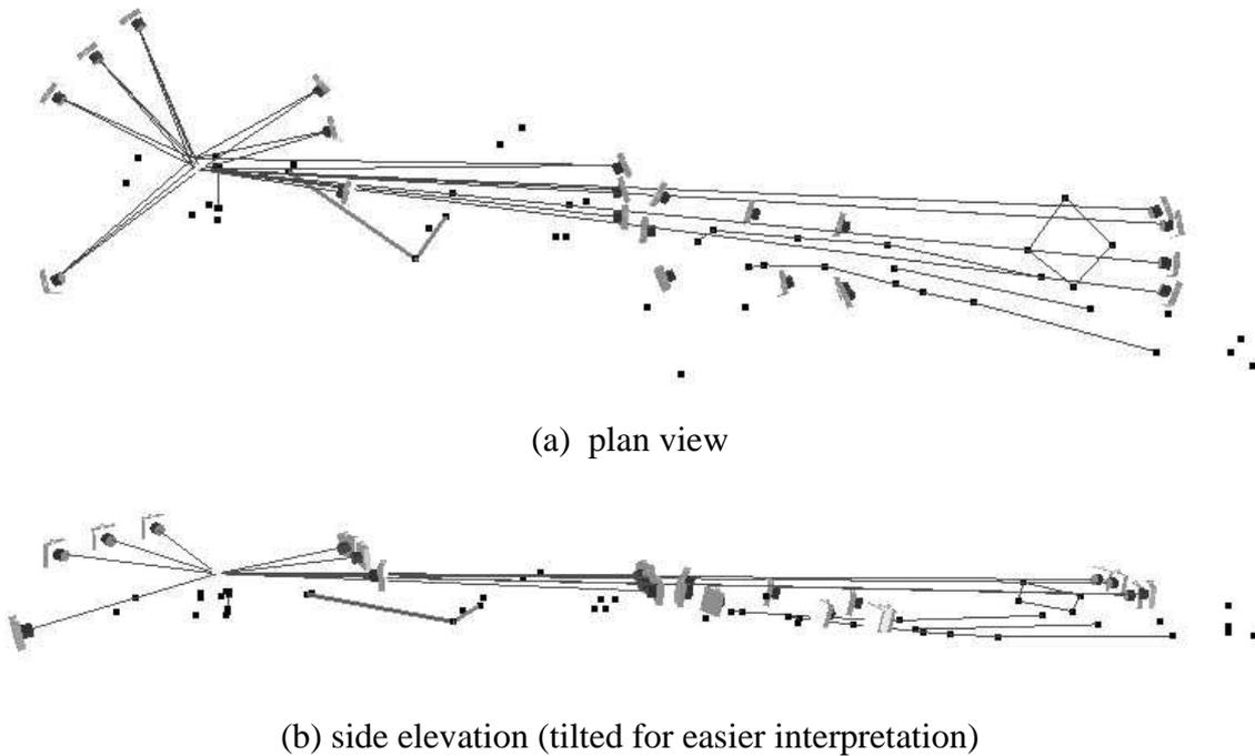
Figure 4: Typical near-planar geometry of photogrammetric networks for AR.
