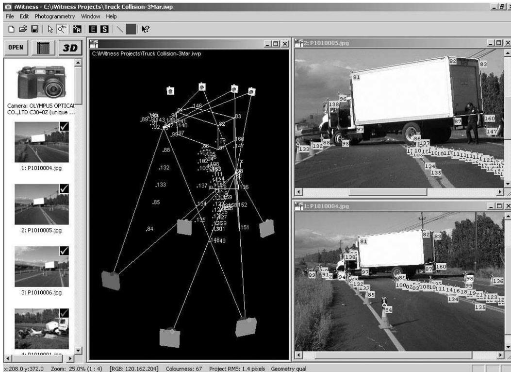
Figure 3: *iWitness* user interface; the CAD diagram in Fig. 1 is from this survey.
