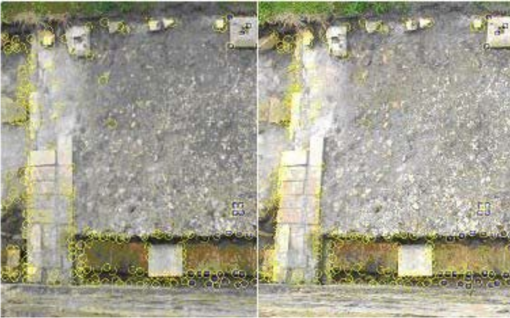
Figure 2: Preparing for image matching by placing conjugate image points around features with large Z variation.
