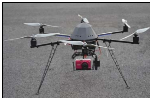
Figure 1. Hexacopter UAV attached with digital camera Canon PowerShot SX230 HS.
