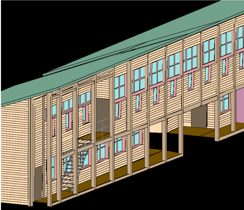
Figure 11: Digital Surface Model in combination with Wireframe Model.
