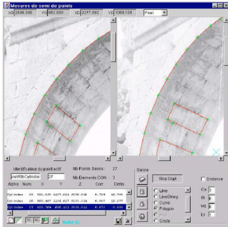
Figure 9. Aleyrac project. Semi-automated Primitive Measurement Method applied to a cylinder shape.
