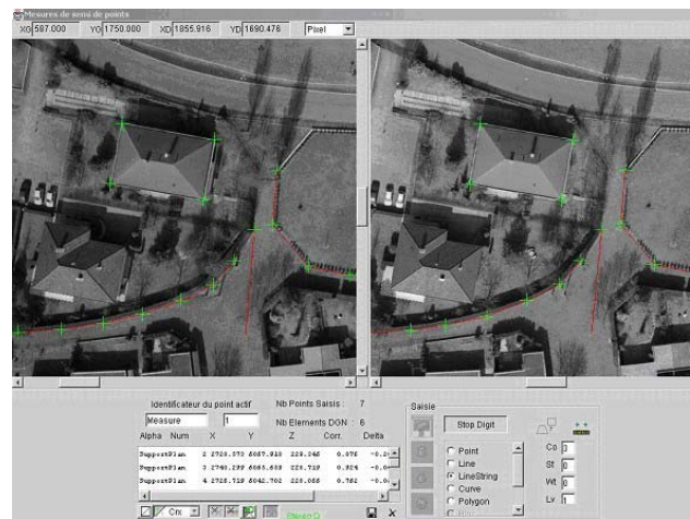
Figure 7. 3D restitution of aerial images
