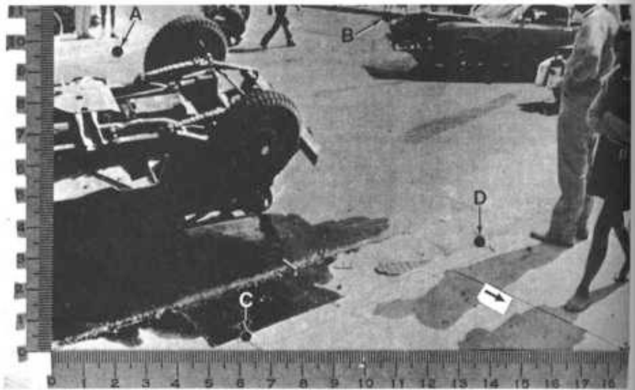
Exhibit 32. With no natural or portable grid available, positions in a photo may be transferred to a map mathematically. The spots must be on a flat surface in the photo. They are located by coordinates. The measured position of at least four spots (A, B, C, and D) on this surface must be visible in the photo and no more than two of them may be in the same straight line.
