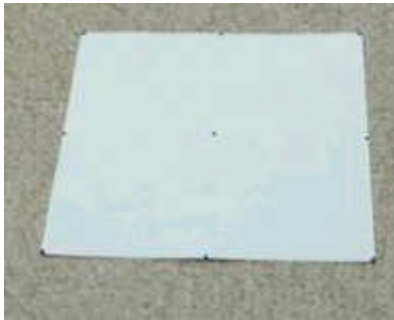
Figure 3: Sample square grid w/ 4 corner points and 4 midpoints. Simply a piece of paper cut square with the points drawn in black.
