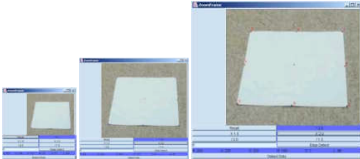
Figure 7: The Zoom Window containing the enlarged "square grid". The last figure shows the Zoom Window with the 8 control points.
