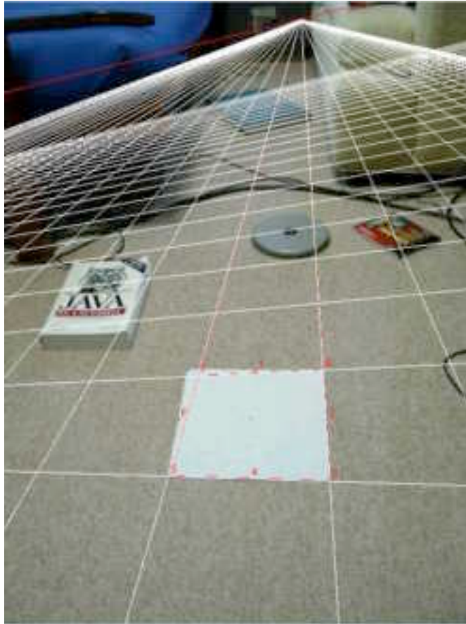
Figure 6: Example of an incorrectly placed control point and its skewed infinite grid.
