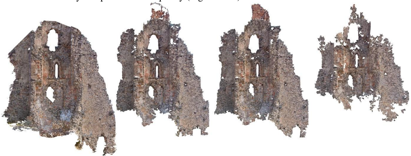
Fig. 2: The preview of the final point clouds of the castle wall; from left – PhotoScan , VisualSFM , OSM-Bundler , Photosynth Toolkit
