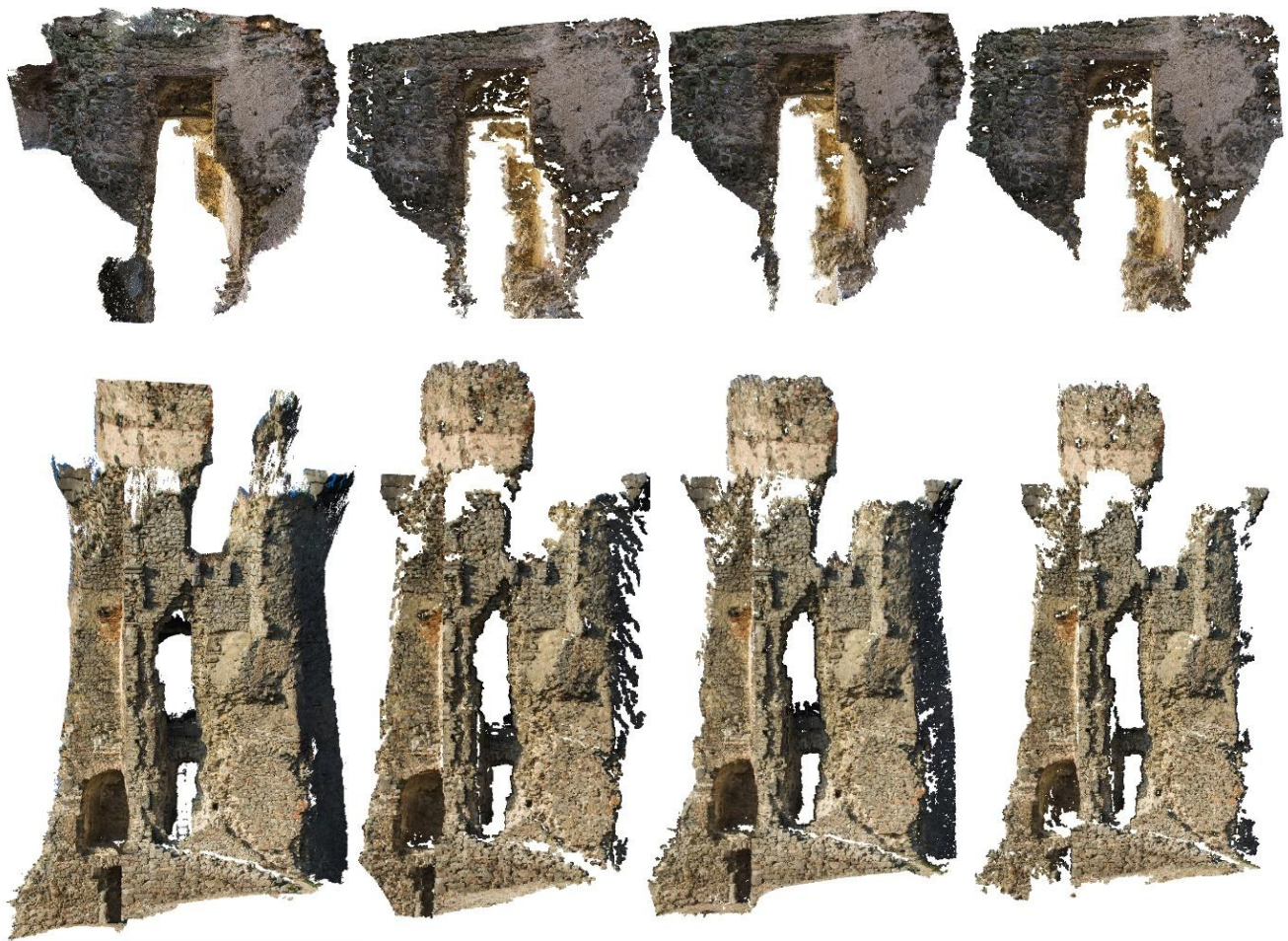
Fig. 3: The preview of the final point clouds of two castle objects; from left – PhotoScan , VisualSFM , OSM-Bundler , Photosynth Toolkit
