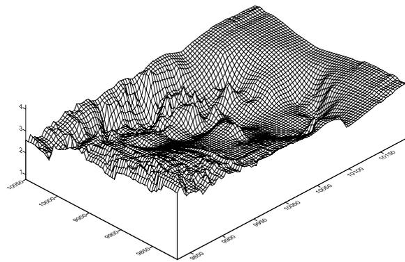
**Figure 9: three dimension map of test area based on photogrammetric methods**
