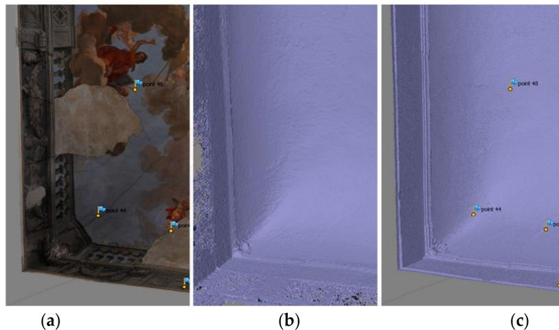
**Figure 1.** (a) Model SfM/LASER; (b) Model SfM/MVS; (c) Model LASER.
