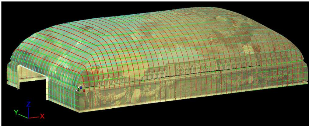
**Figure 2.** Dense contour model (isometric view).
